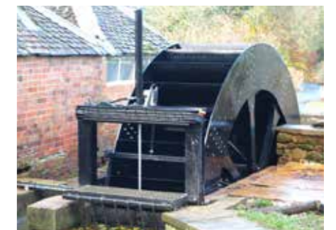
Waterwheel micro hydro scheme
